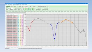
The product will be irradiated with a special developed Halogen lamp. The resulting diffuse reflection (the diffuse reflection contains the necessary information of the constituents) is transmitted via a fibre optic to the spectrometer. The spectrometer split the spectra in 256 support points.
