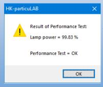
To check the performance of the particuLAB, it is possible to make a performance test with a reference plate.
